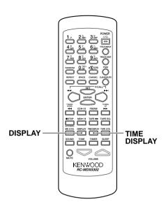
The displayed information switches each time the TIME DISPLAY key on the remote is pressed.
